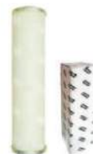
FILTER ELEMENT ID 23 x OD 50 x L 208 mm PARTICLE REMOVAL DOWN TO 15 UM
